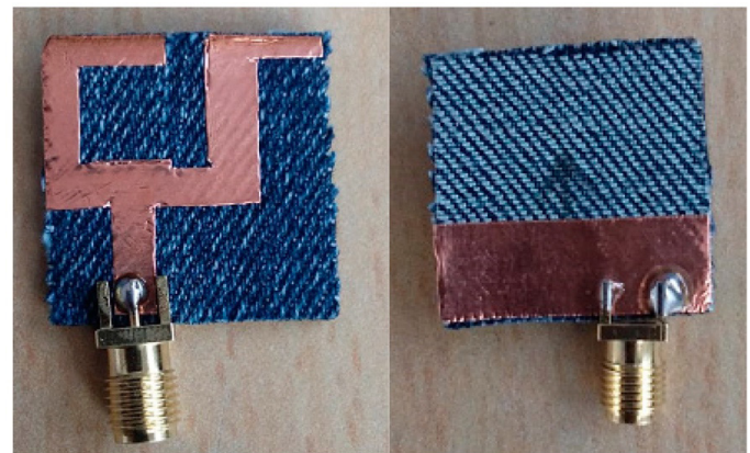
Fig. 1: Wireless Body Area Networks: UWB Wearable Textile Antenna
