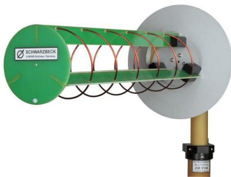
Fig. 2: Helical antenna-II
