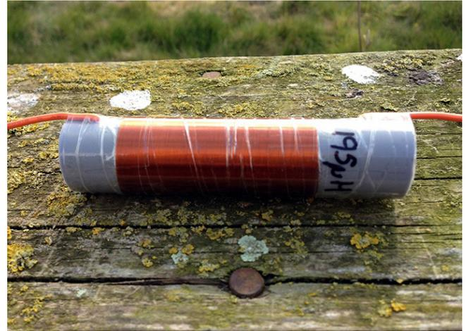
Fig.4: Loaded Quarter Wave Antenna
