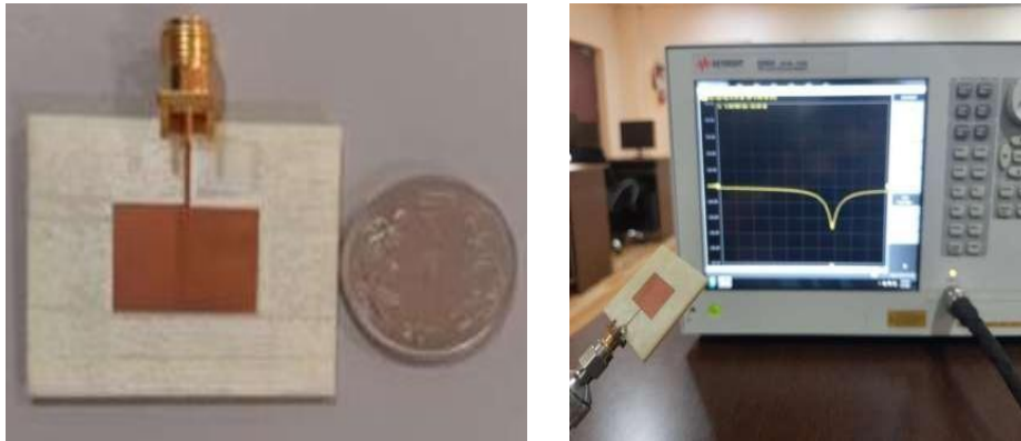
Fig.4: Prototype and measurement setup for dual layer
