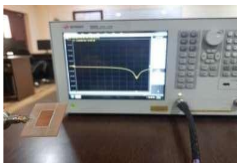
Fig.3: Prototype and measurement setup for single layer
