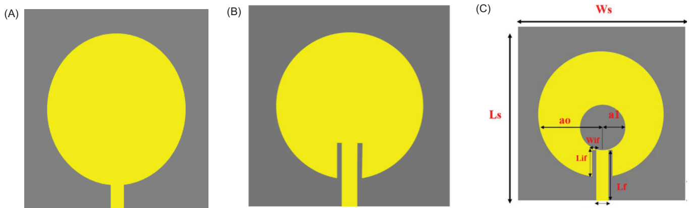
Fig. 1: Basic circular microstrip design (A), with inset-fed addition (B), and antenna with circular slot addition (C).
