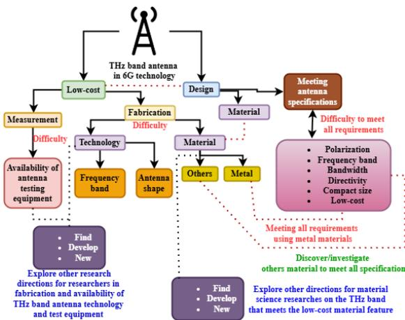
Fig. 3: THz band antenna in 6G wireless communication system.
